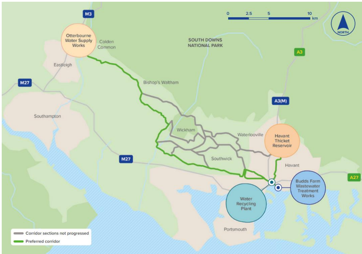
Graphic 3-7 Stage 3 preferred pipeline corridor
