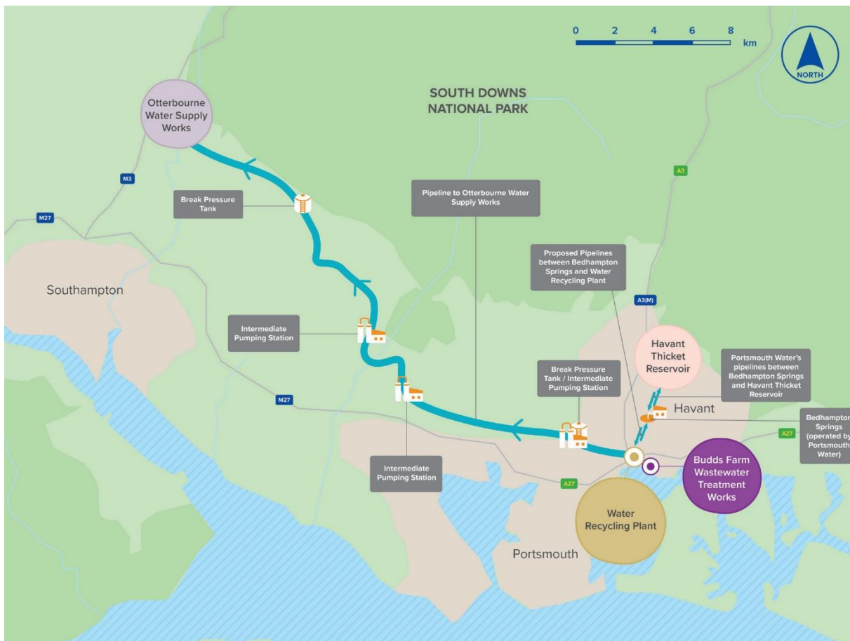
Graphic 2-5 Pipeline between the Water Recycling Plant site and Otterbourne Water Supply Works
